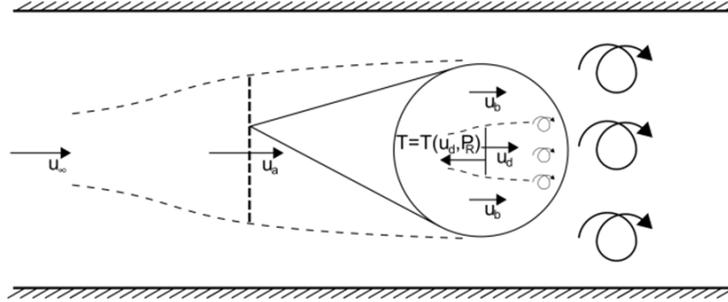
Figure 1: Plan view of a large turbine array, with inset showing flow around individual turbine
