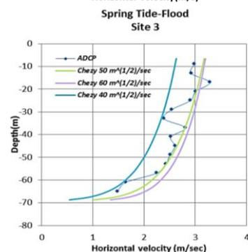
Figure 3: Calibration of flow model inside PF (Site 3)
