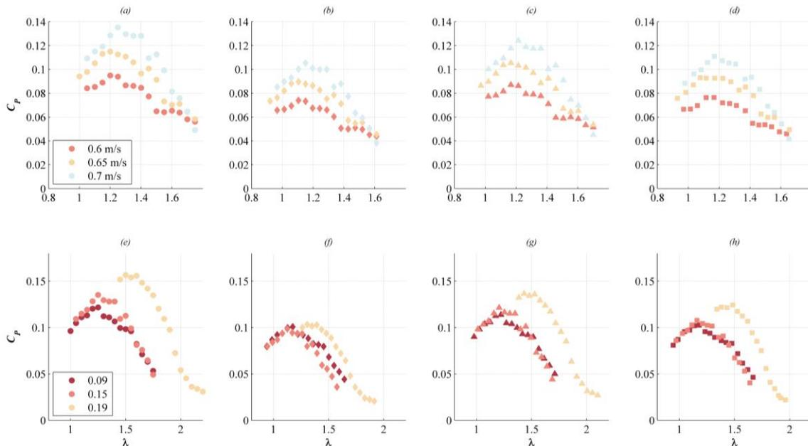
Fig. 1: Performance at same blockage ( $\epsilon = 15\%$ ) varying speed (top). Uncorrected (a) and with Werle, Pope & Harper, and Bahaj et al. corrections (b)-(d), respectively. Performance at same speed (0.7 m/s) varying blockage (bottom). Uncorrected (e) and with Werle, Pope & Harper, and Bahaj et al. corrections (f)-(h), respectively.
