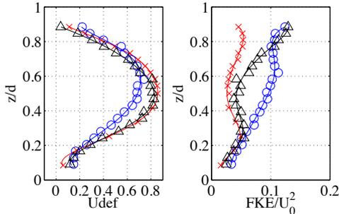
Figure 1: Depth profile of velocity deficit and of kinetic energy of the flow (turbulent and wave induced) measured 2 Diameters downstream of a 3-bladed rotor with thrust coefficient 0.89 and tip speed ratio 5.5. (x - No Wave, o - kd=1 and Δ - kd=3.13)
