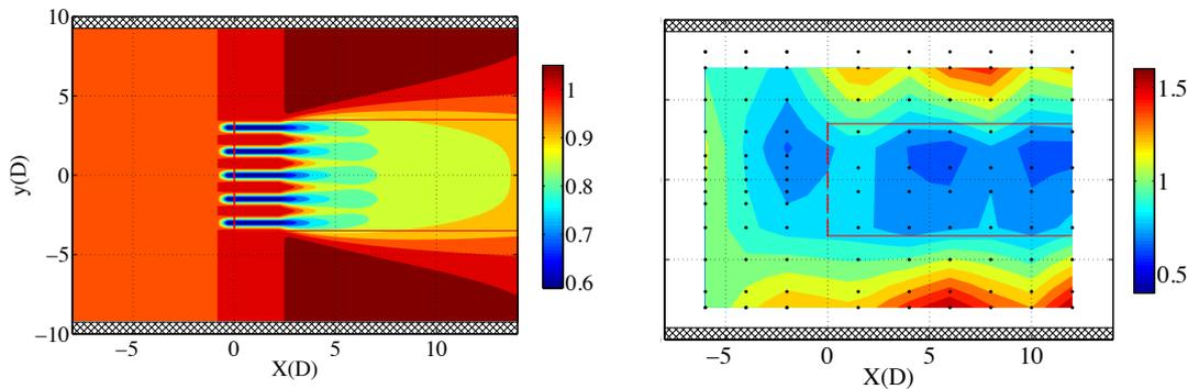
Figure 2: Velocity deficit field (left,  $1-U_x/U_0$ ) from empirical wake model and change of significant wave height (right,  $H_s/H_{s0}$ ) in vicinity of a row of five discs. Disc are at centre to centre spacing of 1.5D with central disc at  $(x,y) = (0,0)$ .
