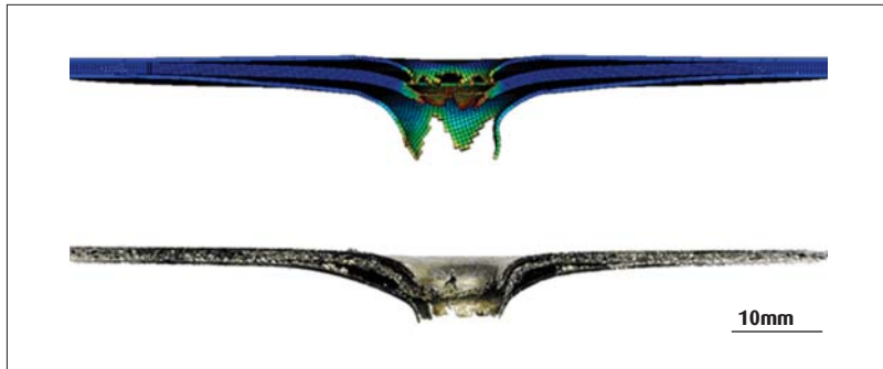
Above: Simulated (top) and actual (below) impact response of sheet. Above far right: Welded box section after compressive overload. Right: Core architecture of sheet obtained using X-ray tomography. Far right: Low-cost honeycomb core produced from 304 stainless steel melt spun fibres
