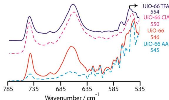
**Fig. 5** IR spectra following the Zr–OC asymmetric stretching vibration of the modulated UiO-66 samples.
