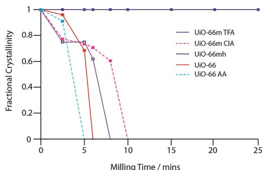
**Fig. 4** Analysis of the crystallinity for various modulated UiO-66 samples as a function of milling time (TFA = trifluoroacetic acid; ClA = chloroacetic acid; AA = acetic acid, mh = modulated removed by heating). Fractional crystallinity is calculated from starting integral breadth/integral breadth at time *t*.
