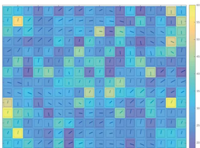
Fig. 5 Mean fibril dimension of fibrils within a single unit cell. Mean fibril dimension was calculated at  $18 \times 14$  positions on the unit cell. For illustration, the orientation distribution indicated by blue bars is superimposed at the location of each scanned image within the map. The colour bar shown on the right indicates the predominant lateral dimension of the scattering objects (average fibril cross-section diameters) in nm.
