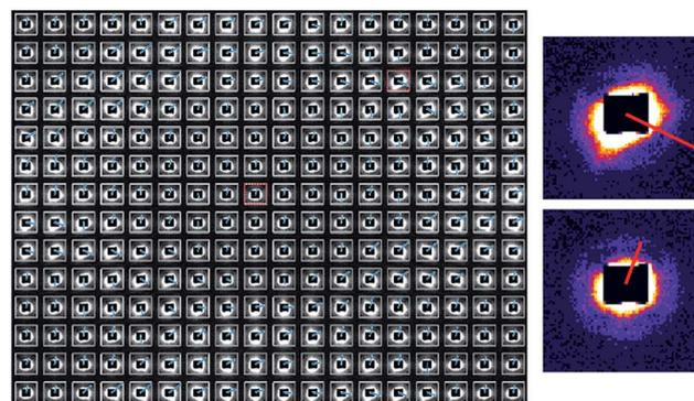
Fig. 4 Orientation distribution of fibrils within a unit cell revealed by SAXS raster scan at  $18 \times 14$  positions. A blue bar on each scanned image indicates the preferred orientation (bar direction) and the degree of alignment (bar length) of fibrils at each position. Two representative patterns, one from the unit cell 'wall' (upper) and one from the cell interior (lower) are shown on the right.
