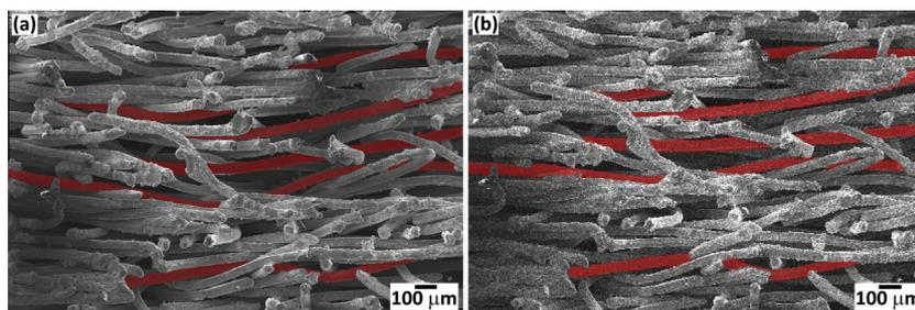
**Figure 2.** Scanning electron microscopy images of a region in the through-thickness face of the 316L fibre networks ( $f = 10\%$ ) showing fibres (some of them highlighted in red) (a) before and (b) after application of an in-plane tensile load (applied horizontally) corresponding to 0.4% strain. (For interpretation of the references to colour in this figure legend, the reader is referred to the web version of this article.)
