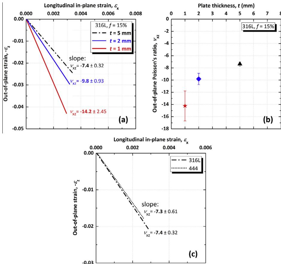
**Figure 4.** (a) In-plane longitudinal strain as a function of out-of-plane strain for 316L fibre networks with  $f = 15\%$ , with three different plate thicknesses; (b) experimental dependence on plate thickness of the out-of-plane Poisson's ratio of 316L fibre networks with  $f = 15\%$ ; (c) in-plane longitudinal strain as a function of out-of-plane strain for 316L and 444 fibre networks with  $f = 15\%$ .
