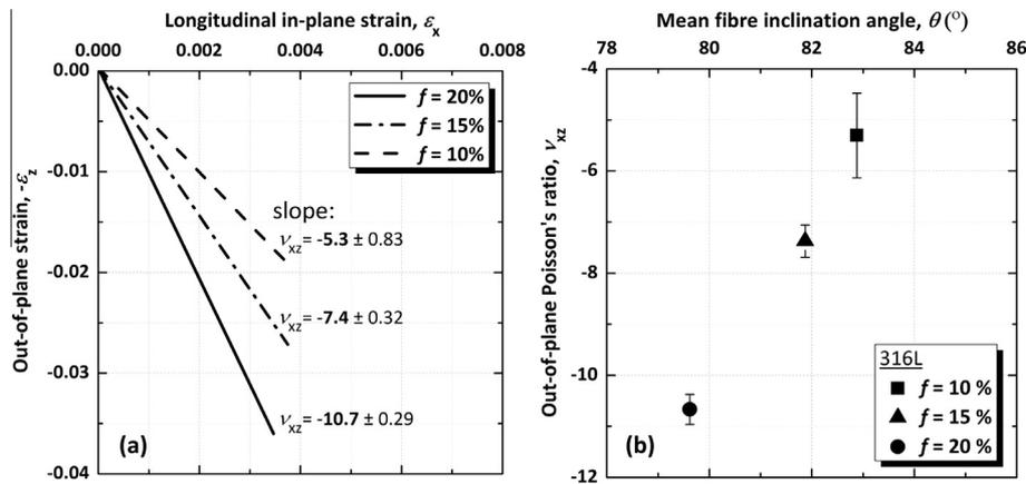
**Figure 3.** (a) In-plane longitudinal strain as a function of out-of-plane strain, measured during in-plane tensile testing of 316L fibre networks, for three different fibre volume fractions [34]; (b) out-of-plane Poisson's ratio plotted as a function of mean fibre inclination angles (with respect to the through-thickness direction), obtained from X-ray tomography, for different fibre volume fractions [34].
