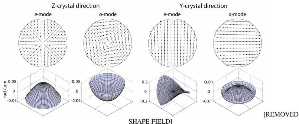
Fig. 2. Polarization eigenmodes for focusing along Z- and Y-crystal direction (top row). The vector diagrams show the polarization profiles of transverse cross-sections through collimated beams. The corresponding phase aberration functions per micron focusing depth are shown below. Both polarization profiles and phase aberrations were calculated for our system parameters.
