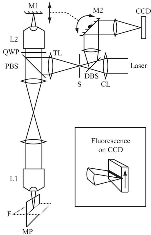
Fig. 1. Slit scanning confocal microscope that images the MP directly with a CCD camera. Inset, line information from different specimen depths is imaged onto different rows of pixels during each frame.
