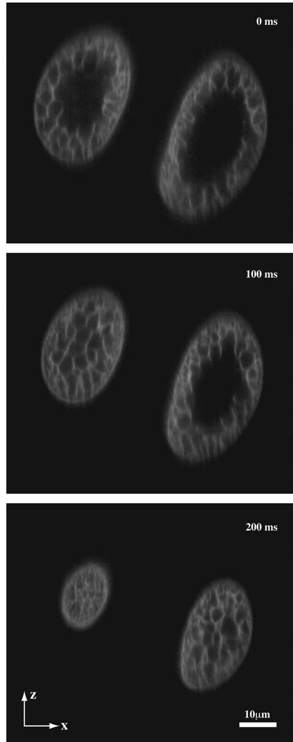
Fig. 2. Image of the parts of a fluorescent pollen grain lying in the MP of our slit scanning confocal microscope. These are frames from a real-time movie obtained of the specimen.
