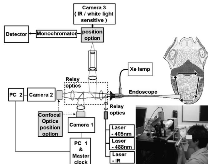
Fig. 3. Schematic representation of the in-vivo video rate confocal endoscopy apparatus. The insert shows the system in use.
