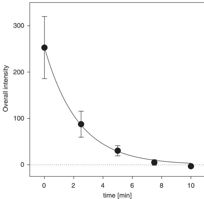
Fig. 11. Example clearance data for a sample of 1.46 wt% CMC in riboflavin-labelled TSS with 25 mM citric acid content. The solid symbols, ●, represent the overall average data and the solid line represents a single exponential fit to the data. The error bars are calculated from the standard deviation in the mean intensity data.
