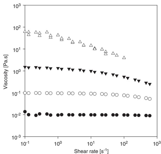
Fig. 1. Steady shear rheology of a solution of CMC in TSS with varying CMC concentration, ● 0.62 wt%, ○ 1.46 wt%, ▼ 2.83 wt% and ▽ 5.50 wt%.
