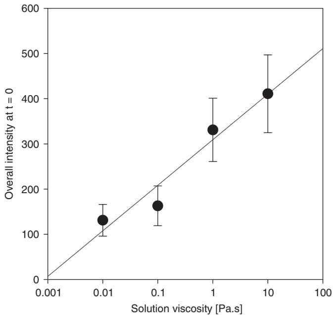
Fig. 8. Plot showing the overall intensities, related to amounts of CMC solution residue remaining on the tongue after oral processing, against viscosity of the solution. The error bars are calculated from the standard deviation in the mean intensity data. The line is a linear fit to the log data as a guide to the eye.
