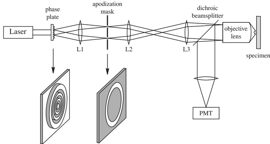
Fig. 6. Schematic diagram of the experimental arrangement. The phase plate is placed in the front focal plane of lens L1 and the apodization mask is located in the back focal plane. Lenses L2 and L3 constitute a  $4f$  system which images the apodized annular illumination into the pupil plane of the objective.
