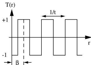
Fig. 3. The phase grating transmission function given in Eq. (9).
