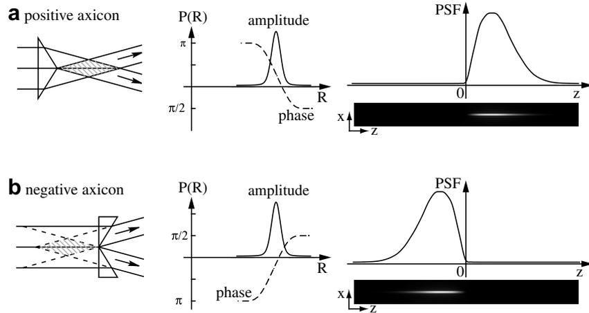
Fig. 2. The pupil function and corresponding intensity profile of the PSF generated by (a) a positive axicon and (b) a negative axicon. Parameters –  $w = 0.5 \text{ mm}$ ,  $t = 25 \text{ mm}^{-1}$ ,  $\lambda = 750 \text{ nm}$ ,  $f = 106.66 \text{ mm}$ ,  $NA = 1.4$  oil immersion.
