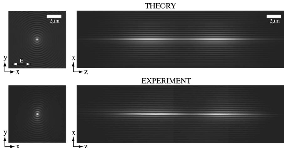
Fig. 7. Numerical simulations (top) and the corresponding experimental images (bottom) generated by scanning a sub-resolution gold bead in the  $XY$  and  $XZ$  planes in reflection mode using annular illumination. See text for parameters used.
