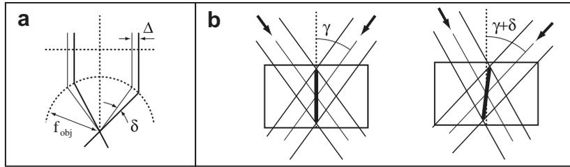
Fig. 10. Laterally shifting the annular pupil function results in a change of parallax angle for the extended PSF. This is shown geometrically in (a) and a closeup of the focal region is shown in (b).
