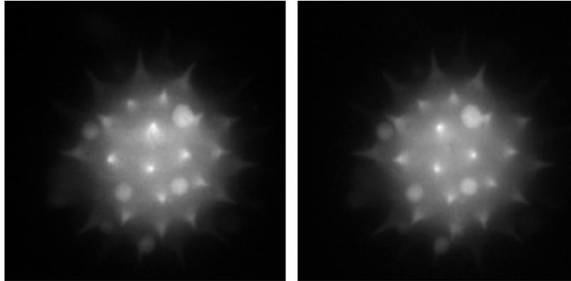
Fig. 11. A stereoscopic image pair taken with an extended depth of focus PSF in two photon fluorescence mode. Line averaging was used to improve the SNR in each.
