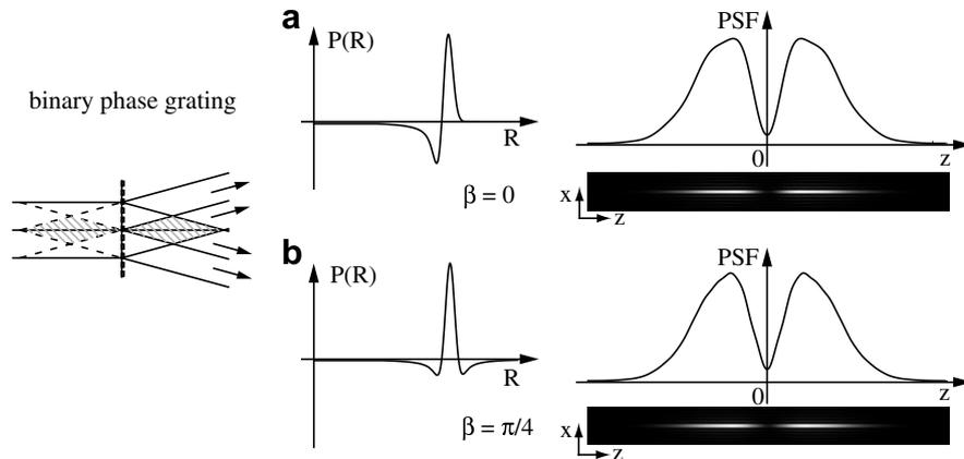
Fig. 4. The pupil function and corresponding intensity profile of the PSF generated by the binary phase grating defined in Eq. (9) with (a)  $\beta = 0$  and (b)  $\beta = \pi/4$ . (Note that the phase variations from each axicon cancel out in the pupil plane to produce a pupil function that is entirely real.)
