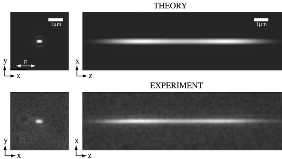
Fig. 8. Numerical simulations (top) and the corresponding experimental images (bottom) generated by scanning a sub-resolution fluorescent polymer bead in the *XY* and *XZ* planes in two-photon fluorescence mode using annular illumination. See text for parameters used.
