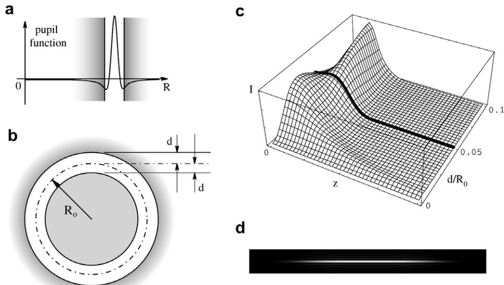
Fig. 5. (a) An illustration of how the apodization mask truncates the field in the pupil plane when  $\beta = \pi/4$ . (b) A further 2D illustration of the same apodization mask and definition of the parameters  $d$  and  $R_0$ . (c) The axial intensity profile of the PSF generated as a function of  $d/R_0$  with the optimally flat PSF marked, (d) the  $xz$  intensity profile of the PSF for this optimal case. (N.B.  $R_0 = t/\lambda f$  gives the approximate position of the peak of the ring.)
