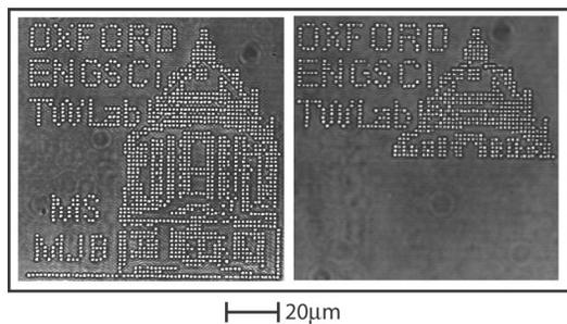
FIG. 3. Transmission images demonstrating aberration correction for recording data. The data were recorded as an array of dots (including a representation of the Radcliffe Camera building in Oxford). Left—correction on during the whole writing process. Right—for the second half of the writing process the aberration correction was switched off.
