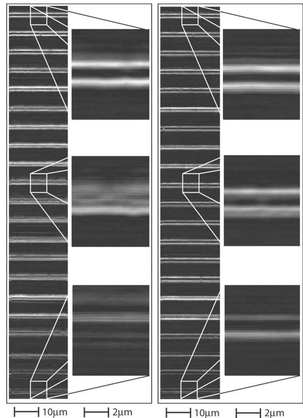
FIG. 2. Axial section confocal microscope scans of the whole multilayer recording medium with detail shown for the 1st, 10th, and 20th layers. The aberration correction was fixed at the level required for the top layer (left) and adapted for each individual layer (right). The optical axis is oriented down the page in these images.
