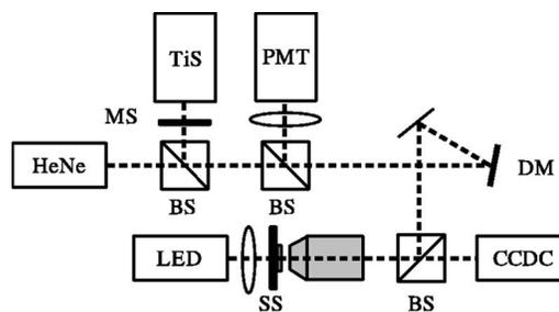
FIG. 1. Schematic of the experimental system. Some intermediate lenses have been omitted for clarity. Key: HeNe—helium-neon laser, Ti:S—titanium-sapphire laser, PMT—photomultiplier tube, DM—deformable mirror, CCDC—CCD camera, BS—beam splitter, MS—mechanical shutter, SS—scanning stage.
