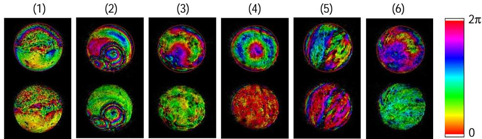
Fig. 3. Specific interferogram examples from a particular position within the  $16 \times 16$  grid that was recorded for each specimen. The color encodes the phase, the brightness corresponds to the amplitude. The numbers (1) to (6) are the specimen numbers listed in Table 1; The upper part shows the measured initial wavefront, the lower part a simulated correction of the Zernike modes up to  $i = 22$ .
