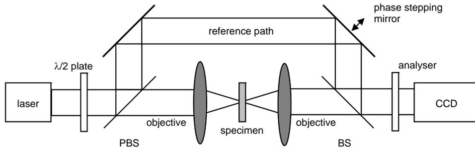
Fig. 1. Phase stepping interferometer for aberration measurement (see text). (PBS - polarising beam splitter, BS - beam splitter.) The specimen is mounted between two opposing high NA lenses and scanned laterally by means of a computer controlled stage. Some intermediate lenses have been omitted for clarity.
