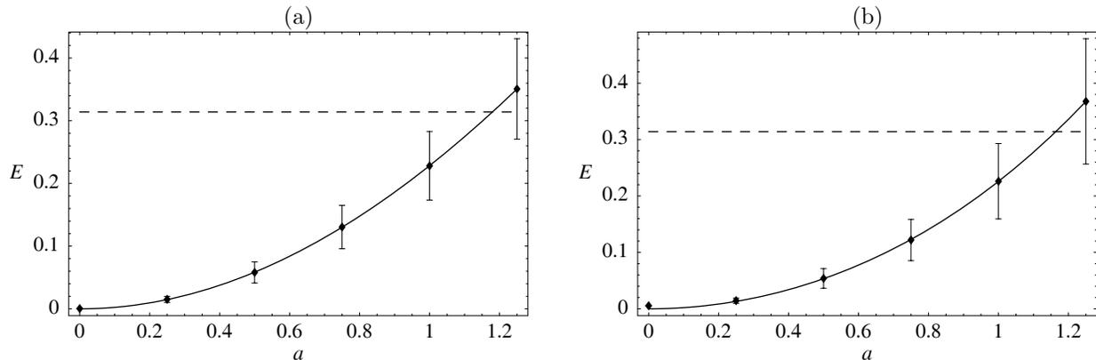
**Figure 5.** Measurement accuracy of multiple mode, simplex biased MWFS configurations as a function of input aberration vector magnitude. (a) for modes 5, 6, and 11 with  $b_{max} = 0.5$ . (b) for modes 4 to 8 with  $b_{max} = 0.5$ . The data points show the mean and standard deviation using a sample of 1000 input wave fronts. The solid line is a fourth order even polynomial fit. The dashed line shows the measurement tolerance of  $\pi/10$ .
