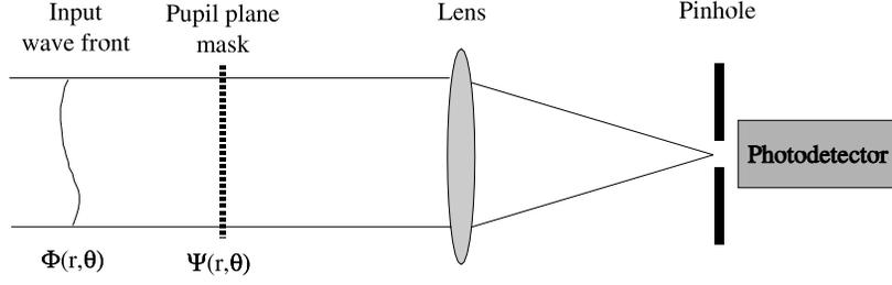
**Figure 1.** Schematic diagram of the wave front sensor measurement system. The input wave front is incident from the left whereupon it passes through the pupil plane of the lens. A phase element in this plane adds a chosen phase aberration to the input wavefront. The wave front is then focussed by the lens onto pinhole positioned at the nominal focus where the intensity signal is measured by the photodetector.
