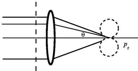
**Fig. 3** The use of radially polarized light results in a purely axially polarized electric field at the geometrical focus. A point scatterer located at focus radiates as a dipole with a far-field pattern (dashed lines).
