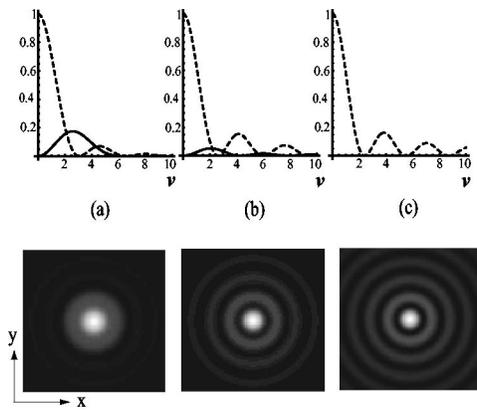
**Fig. 2** Relative strengths of the lateral (solid line) and axial (dashed line) components of the electric field in the focal plane of an objective lens, NA=1.0: (a) no apodization; (b) and (c) 80% and 99% annular apodization, respectively; (d), (e), and (f) corresponding form of the focal spot  $|E|^2$ .
