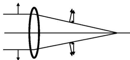
**Fig. 1** Schematic diagram showing the electric field components of a radially polarized beam when it is focused by an objective lens.
