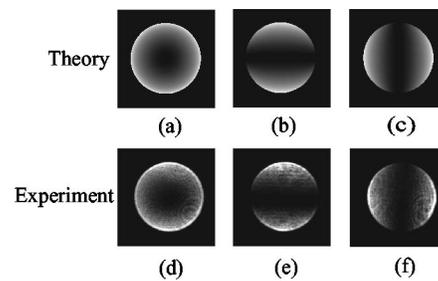
**Fig. 4** (a) and (d) Theoretical and experimental back focal plane intensities. (b), (e) and (c), (f) The vectorial nature of the field is revealed with the aid of “horizontal” and “vertical” linear polars, respectively. The objective used was a 63X, 1.4-NA oil immersion objective and a 0.532- $\mu\text{m}$  laser was used as the light source.
