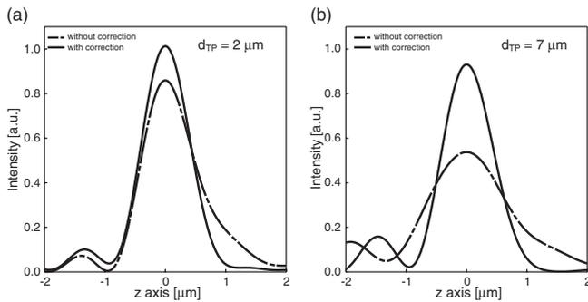
Fig. 3. Intensity distributions along the optical axis with and without the aberration correction for (a)  $d_{TP} = 2 \mu\text{m}$  and (b)  $d_{TP} = 7 \mu\text{m}$ . Solid line; with the aberration correction, broken line; without the aberration correction.
