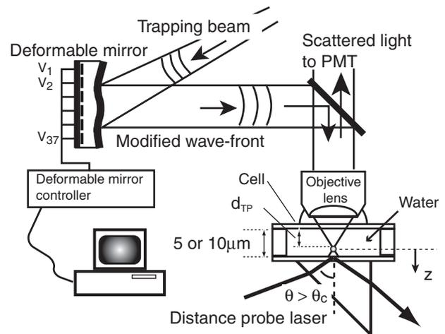
Fig. 1. Experimental setup for laser trapping with aberration correction system and for measuring the spring constant.
