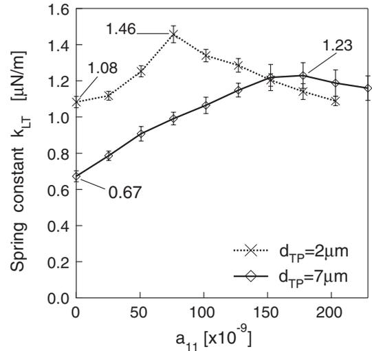
Fig. 2. Spring constants with aberration correction as functions of the magnitude of the 11th order polynomial  $a_{11}$ . ( $\times$ )s with a dashed line are for  $d = 2 \mu\text{m}$  the spring constants and ( $\diamond$ )s with a solid line are for  $d = 7 \mu\text{m}$ .
