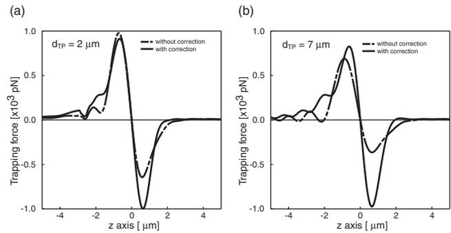
Fig. 4. Trapping forces on a 1- $\mu\text{m}$  diameter-polystyrene particle in the incident fields with and without the aberration correction at (a)  $d_{TP} = 2 \mu\text{m}$  and (b)  $d_{TP} = 7 \mu\text{m}$ . Solid line; with the aberration correction, broken line; without the aberration correction.
