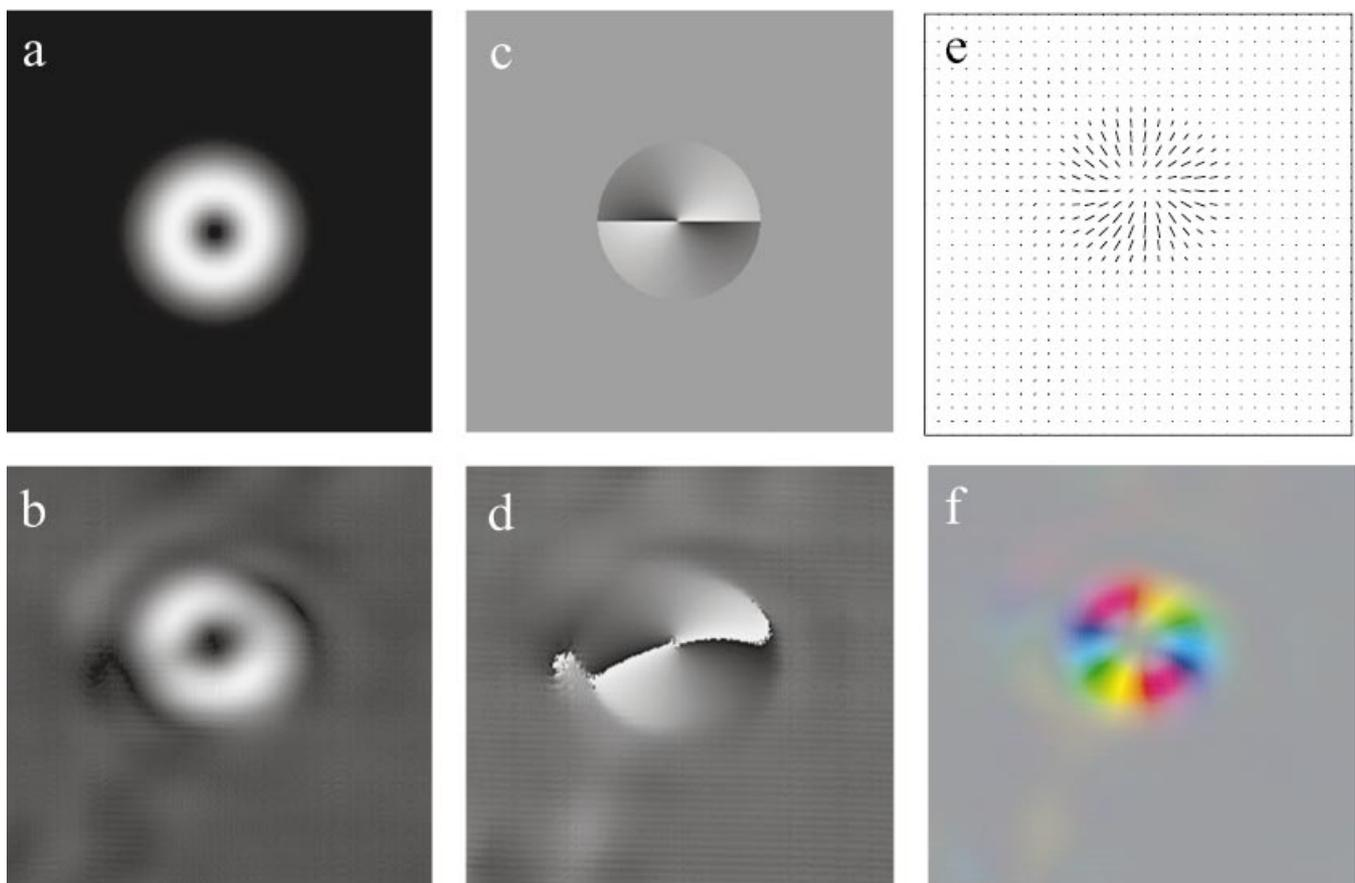
**Fig. 10.** A comparison between theory and experiment in the imaging of a point scatterer. (a) and (c) show the theoretically predicted magnitude and orientation images together with the experimental confirmation in (b) and (d), respectively. Combined experimental polarization images are shown in (e) and (f) using the two alternative representations previously introduced.
