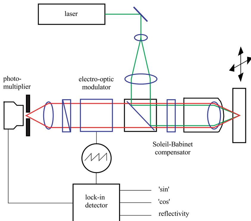
Fig. 2. Schematic diagram of the optical configuration of the polarization contrast confocal microscope. The Soleil-Babinet compensator, set to act as a quarter wave plate, is used both to launch circularly polarized light into the optical system and also as the first element in the electro-optic rotating analyser. The lock-in amplifier detects the two quadrature components from which the magnitude of the optical anisotropy as well as the orientation can be extracted.
