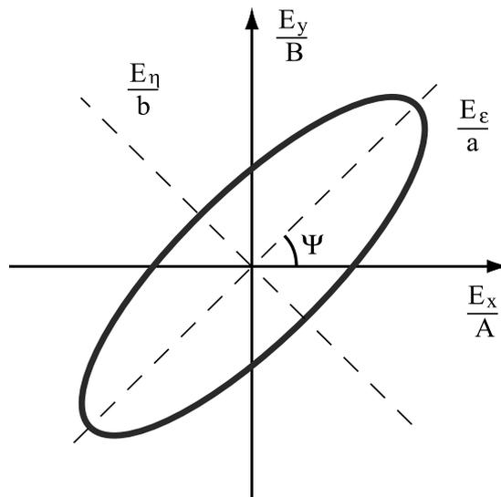
Fig. 1. The polarization ellipse indicating the general state of polarization of an arbitrary input beam. The length of major and minor axes of the ellipse with respect to its principal axes are  $2a$  and  $2b$ , respectively.
