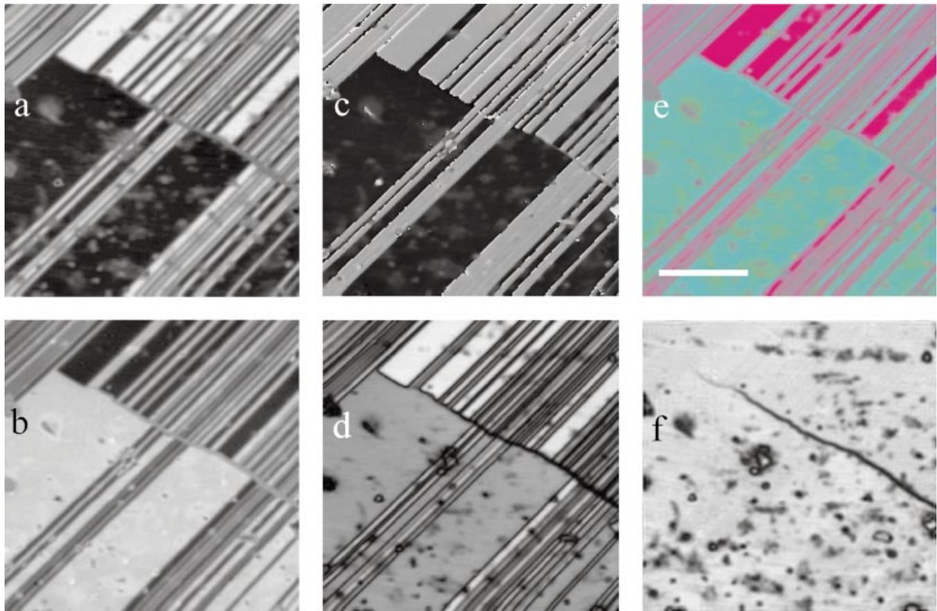
**Fig. 5.** Images of a section of the superconducting crystal  $\text{Y}_1\text{Ba}_2\text{Cu}_3\text{O}_{6.94}$ . (a) and (b) show the two quadrature demodulated signals from the lock-in detector from which the orientation (c) and magnitude (d) images are derived. These two images may be combined into a single colour-coded polarization contrast image (e) using the colour mapping of Fig. 4. Finally, a reflected light confocal image (f) is presented. The scale bar represents 5  $\mu\text{m}$ .
