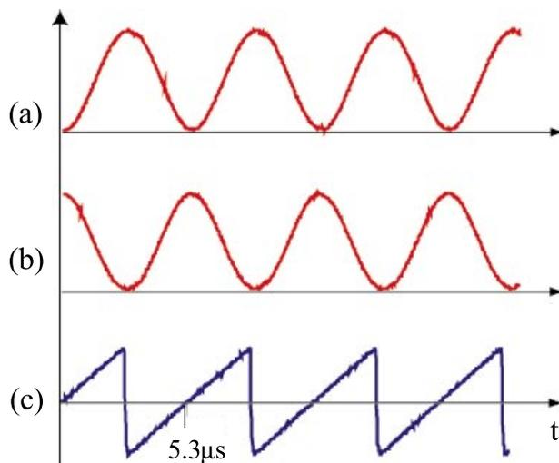
Fig. 3. Experimental confirmation of the operation of the electro-optic implementation of the rotating analyser. The lower trace (c) shows the saw-tooth waveform which is used to sweep the retardance of the Pockels cell. The upper two traces show the measured intensity transmitted when the incident light is (a) vertically and (b) horizontally polarized.
