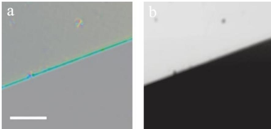
**Fig. 9.** Polarization (a) and reflected light confocal (b) images of a cleaved edge of indium phosphide. The images show both the effects of edge scattering as well as the polarization images to be expected from a point scatterer. The scale bar represents 5  $\mu\text{m}$ .
