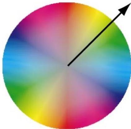
**Fig. 4.** The colour map used to encode the state of polarization of the light reflected from the sample. The direction of the arrow denotes the orientation of the principal axis of the ellipse via the hue of the colour, whereas the saturation, radial distance, encodes the ellipticity. The centre of the circle corresponds to unit ellipticity (circular polarization), whereas the edge denotes minimum ellipticity present in the image. The same colour-coding scheme is used in all the figures.
