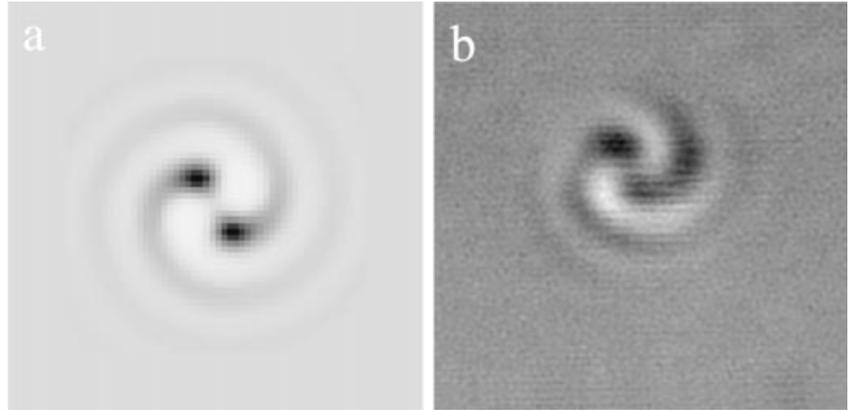
**Fig. 11.** The effect of defocus is illustrated by comparing the theoretical (a) and experimental (b) demodulated images for a defocus value corresponding to  $kz = 5$ .
