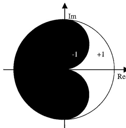
Fig. 1. Mapping of a normalized complex field within a unit circle into the required +1 or -1 modulation of the binary optical element.
