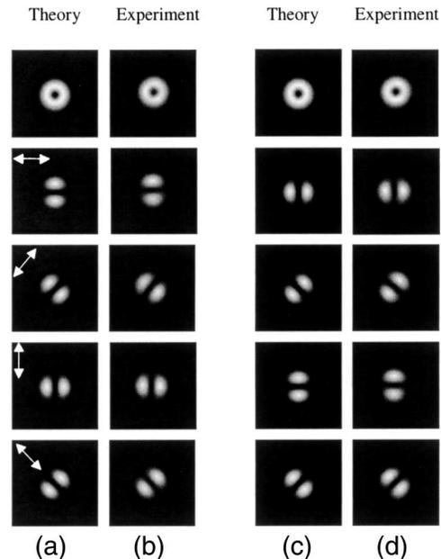
Fig. 3. Intensities in the focal plane comparing theory, (a) and (c), with experiment, (b) and (d), for both azimuthally, (a) and (b), and radially, (c) and (d), polarized illumination. The top row shows the full intensity, whereas the rows below reveal the vectorial nature of the field by showing the intensity passed by an analyzer oriented as indicated by the arrows.
