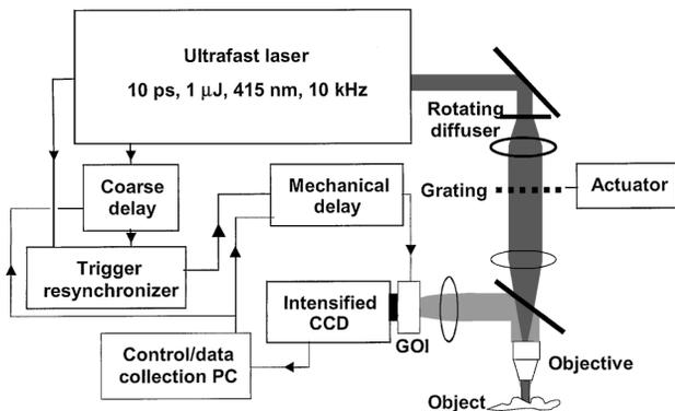
Fig. 1. Experimental setup for whole-field 3-D fluorescence lifetime imaging by use of structured light. GOI, gated optical intensifier.
