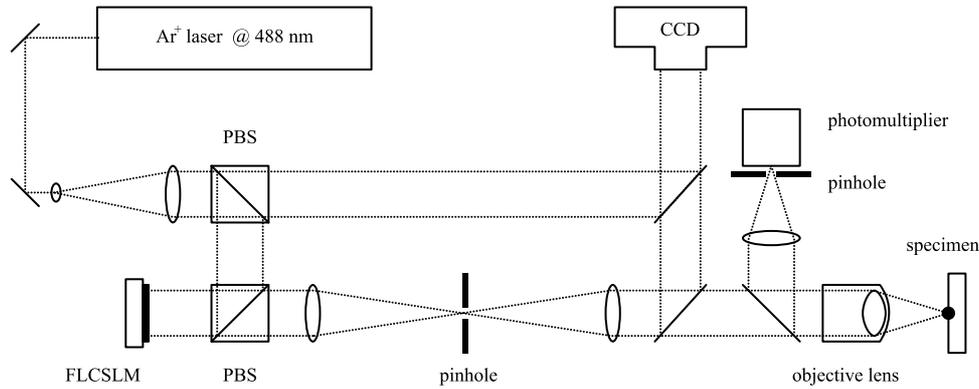
Fig. 3. Schematic diagram showing both the wavefront generator and its interface to the microscope system. PBS = polarizing beamsplitter; FLCSLM = ferroelectric liquid crystal spatial light modulator.
