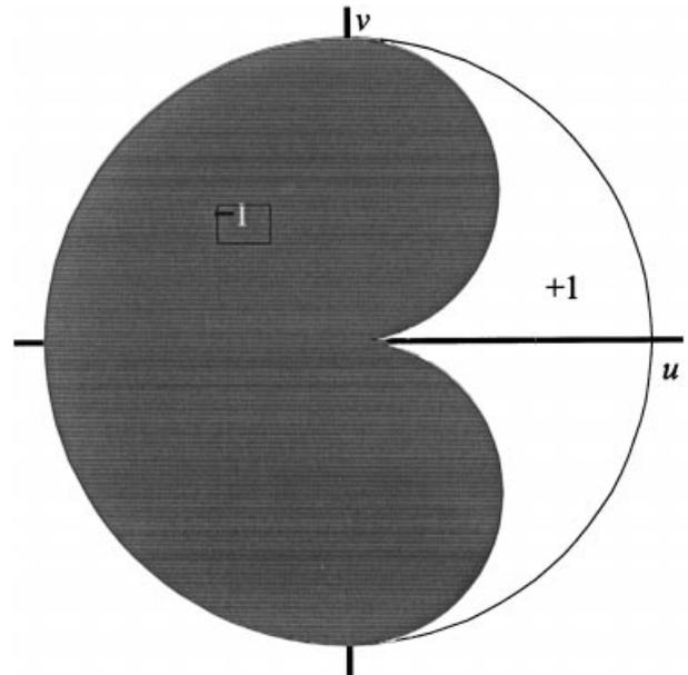
Fig. 2. The mapping of a complex field  $u + jv$  into the required  $+1$  or  $-1$  phase modulation.
