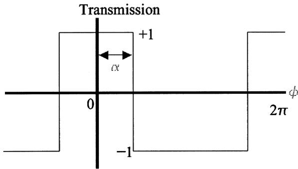
Fig. 1. The binarizing scheme showing that the transmission of the binary optical element is determined by the phase together with the angle,  $\alpha$ .
