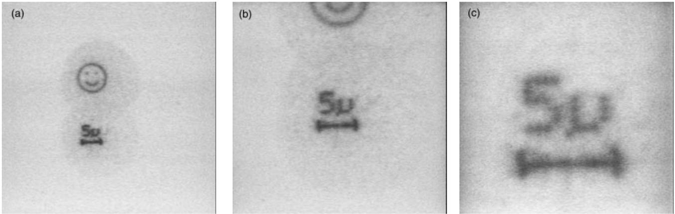
**Fig. 5.** Confocal images of a fluorescent sheet. The scale bar and other image details were photobleached into the specimen by the wavefront generator.
