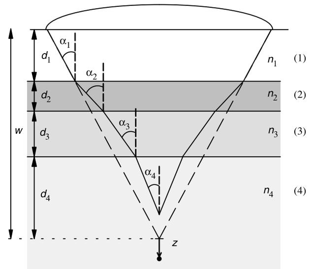
Fig. 2. Schematic diagram of the focusing geometry for the confocal imaging of skin. Layer (1) is the lens immersion medium. The skin is approximated by the three-layer structure shown, consisting of (2) the stratum corneum (3) the epidermis, and (4) the dermis.
