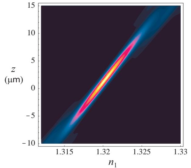
Fig. 8. Confocal axial response for focusing with an NA = 0.9 water immersion lens to a depth  $d_4 = 200 \mu\text{m}$ . The immersion medium used has a refractive index  $n_1$  as shown on the horizontal axis.
