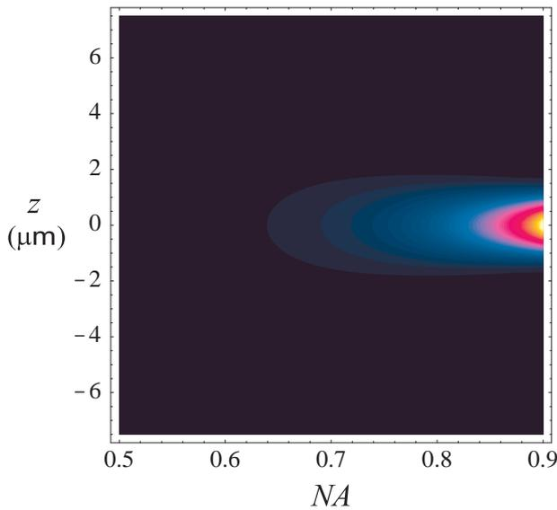
Fig. 6. Confocal response to an on-axis point object in a refractive index matched medium ( $n = 1.33$ ) as a function of numerical aperture for a water immersion lens of nominal NA = 0.9.
