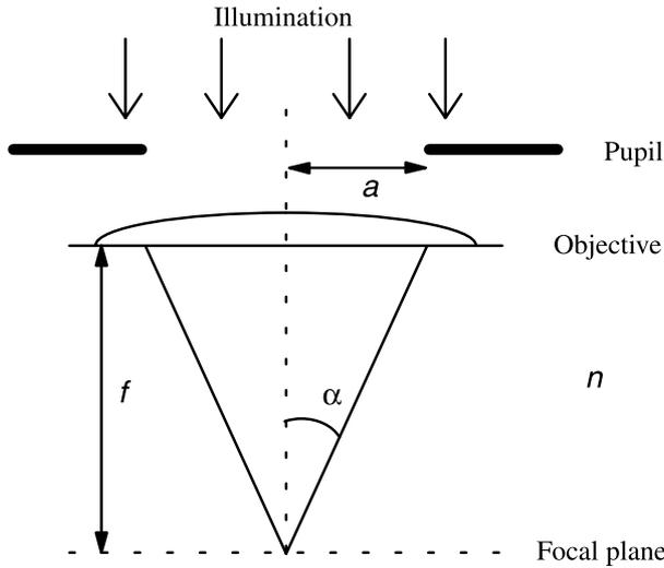
Fig. 1. Schematic showing the focusing geometry of the objective lens. The adjustable circular pupil has radius  $a$  and is illuminated by a constant power density.
