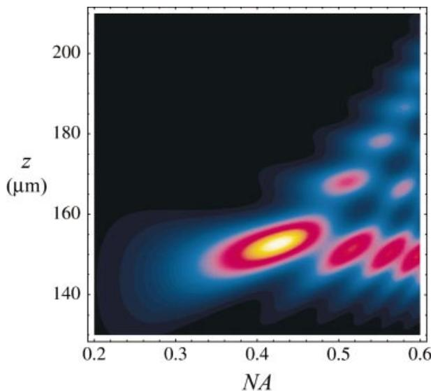
Fig. 4. Confocal response to an on-axis point object as a function of numerical aperture for a dry lens of maximum NA = 0.6. The depth  $d_4 = 200 \mu\text{m}$ . The illumination has been adjusted so that the same total power passes through the pupil for all NA.
