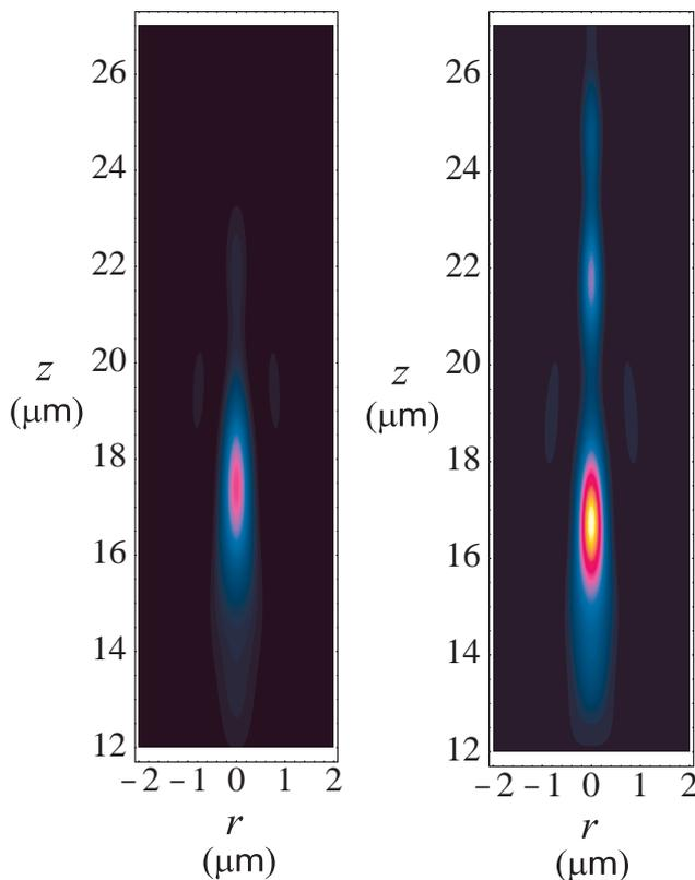
Fig. 7. Confocal point spread function cross-section plots using a water immersion lens focusing at a nominal depth  $d_4 = 200 \mu\text{m}$  for (a) NA = 0.77 and (b) NA = 0.9.
