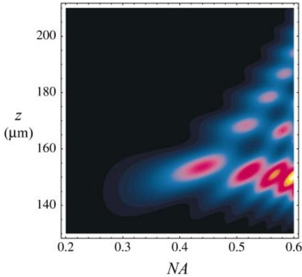
Fig. 3. Confocal response to an on-axis point object as a function of numerical aperture for a dry lens of maximum NA = 0.6. The depth  $d_4 = 200 \mu\text{m}$ . The colour table shows signal level normalized to the maximum value in this plot.
