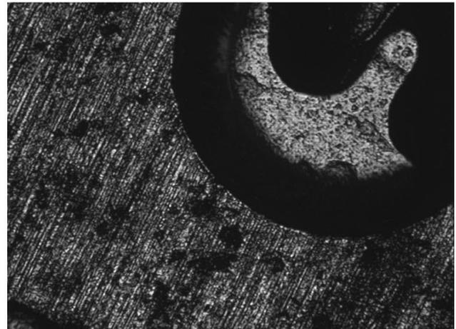
Fig. 2. Optically sectioned images, taken at focal settings 1.25 mm apart, of a section of a wrist watch mechanism: the scale bar depicts a length of 100  $\mu\text{m}$ .
