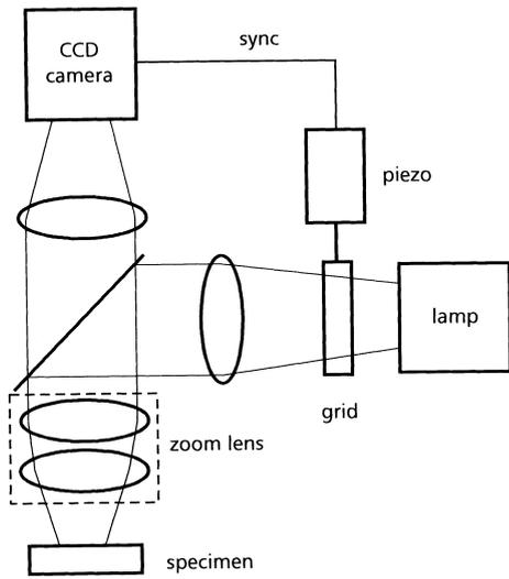
Fig. 1. Schematic diagram of the macroscope system.
