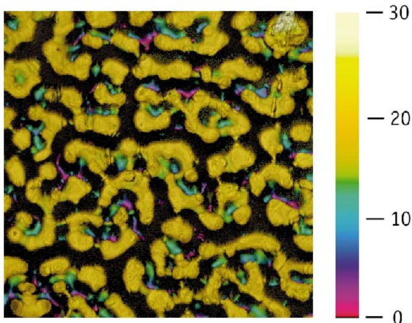
Fig. 2. A colour-coded height representation of Fig. 1(b). The height scale on the right of the image is in micrometres. Both reflectivity and height are encoded in the image as brightness and hue, respectively.
