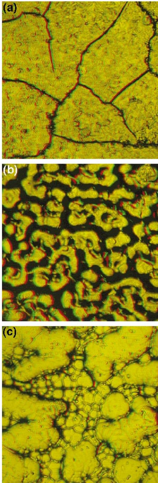
individual confocal images. In all three cases the light intensity provided by the projector lamp was more than sufficient to produce reflectance images of high signal-to-noise ratio. These 3D images show the wide range of microscopic surface morphology found in combustion chamber deposits. The surface morphology of these deposits is influenced by temperature gradients in the combustion chamber, the chemical composition of the fuel and the running conditions of the engine.
