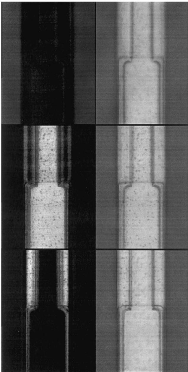
**Fig. 4.** A through-focus series of a portion of a semiconductor wafer. The left-hand column represent the optically sectioned images whereas the right-hand column shows the corresponding confocal images. The images were taken at focal settings  $0.8\ \mu\text{m}$  apart using a  $100\times$ ,  $0.95\text{-NA}$  Olympus MPlanApo objective lens. The image size is  $43\ \mu\text{m} \times 57\ \mu\text{m}$ .
