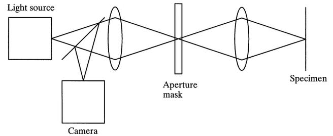
Fig. 2. Schematic diagram of the microscope system.
