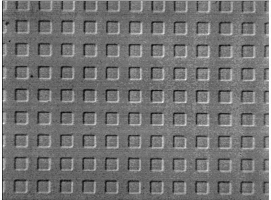
**Fig. 5.** A Normarski differential interference contrast image of 5- $\mu\text{m}$  square phase islands within a semiconductor test pattern. The images were taken with a 50 $\times$ , 0.7-NA Olympus Neo SPlan objective lens and the image size is 115  $\mu\text{m}$   $\times$  86  $\mu\text{m}$ .
