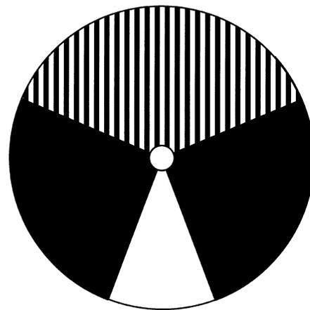
Fig. 3. Schematic diagram of the aperture mask showing the orientation of the grid lines.
