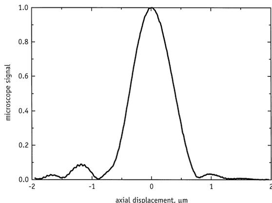
Fig. 2. The measured axial response of the system.
