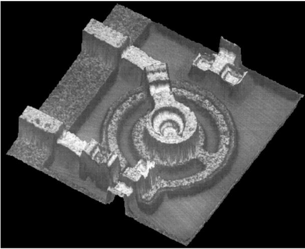
Fig. 3. Three-dimensional image of a transistor. The height projection image is combined with an autofocus image to provide surface rendering. A  $50\times/0.8$  numerical aperture objective was used. The image field is  $120\ \mu\text{m} \times 120\ \mu\text{m}$ .
