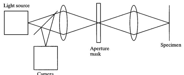
Fig. 1. Schematic diagram of the confocal microscope.
