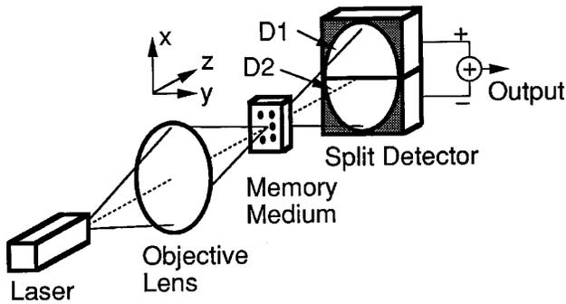
Fig. 1. Optical setup for a phase-contrast microscope with a split detector.
