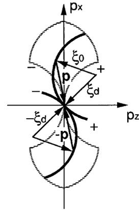
Fig. 2. Calculation process for the derivation of the 3-D transfer function. The two opposing arcs at the origin of the  $(p_x, p_z)$  coordinate, indicated by dashed curves, are the 3-D optical transfer functions for a phase object with coherent detection. The two arcs indicated by the heavy curves are also 3-D optical transfer functions for the point detector located at  $(\xi_d, \zeta_d)$ .
