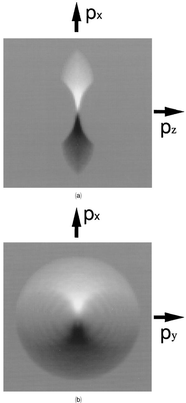
Fig. 3. 3-D OTF: (a) cross section of the  $p_x$ - $p_z$  plane, and (b) cross section of the  $p_x$ - $p_y$  plane.
