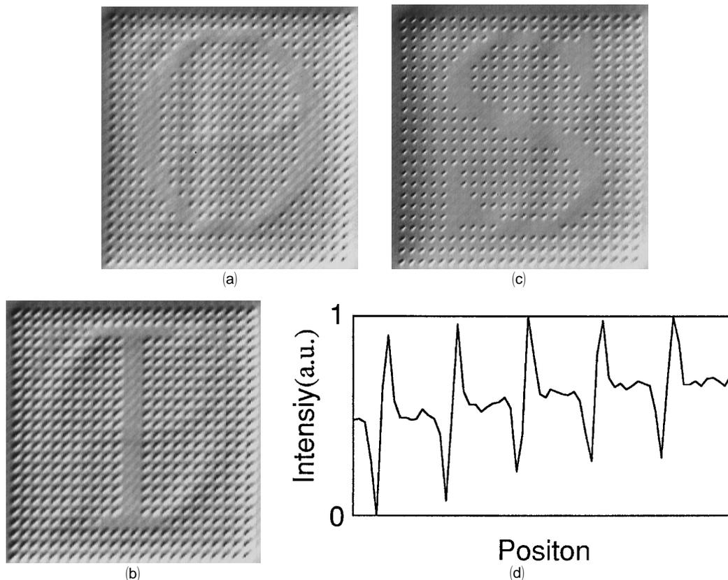
Fig. 4. Experimental results of the readout of the data: (a) the first layer, O in a square is formed by the bit sequence; (b) the fourth layer, formed with I; (c) the sixth layer, with S; and (d) a cross section of 5 bits along the diagonal of (c).
