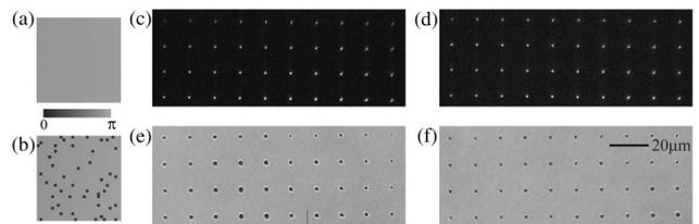
Fig. 3. Active region of the SLM corresponding to a single microlens with a flat phase profile and (a) a  $\pi$  phase shift introduced to a random selection of pixels to reduce the focal intensity by 10%. (b) Images of the array of foci before and (c) after (d) the homogenization process. The resultant fabrication is seen on the surface of fused silica without and (e) with (f) homogenization of the microlens array.
