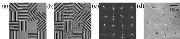
Fig. 4. Phase pattern applied to the SLM to variably steer individual lenslet foci and create a  $4 \times 4$  aperiodic array of foci, before and (a) after, (b) taking into account the SLM beam steering inefficiency. The associated focal intensity distribution and surface ablation are shown in (c) and (d), respectively.
