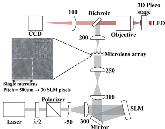
Fig. 1. (Color online) Experimental setup for addressable multispot micromachining. The inset shows an image of a  $2 \times 2$  segment of the microlens array mapped onto the SLM (a binary phase checkerboard is applied to the region of the SLM corresponding to the top right lenslet).
