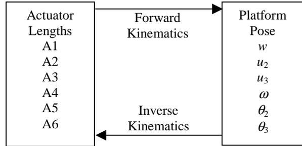
Figure 5: Calculation procedures used in computer program.
