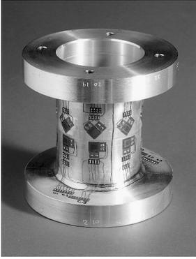
Figure 6: The 6 degree-of-freedom load cell.
