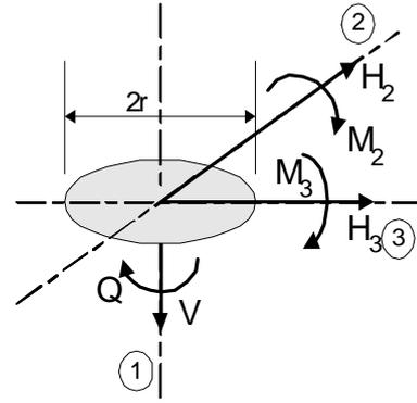
Figure 3: 6dof loading on a circular foundation.
