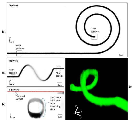
FIG. 3. Examples of single wires following spiral and helical paths. Both wires were fabricated with four axially shifted passes of the laser beam. The depth of the helical wire ranged from 10 to 30  $\mu\text{m}$ . The positions of subsequent pillar fabrication are marked in the images. (a) Optical transmission microscope image of the spiral wire. (b) Top view and (c) side view of helical wire. (d) 3D SHG microscope image of the helical wire.
