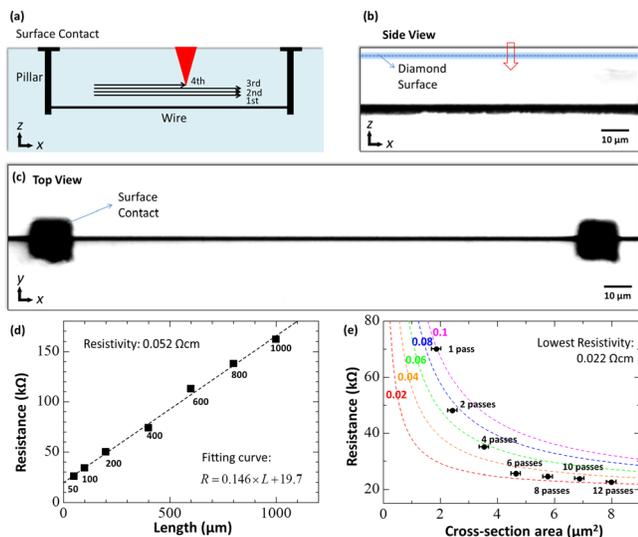
FIG. 2. (a) Sketch of axial multi-fabrication scheme, and the structure of embedded wire contacts and pillars. (b) Side view and (c) top view optical microscope images of the wire for resistance measurement. (d) Resistance as a function of the wire length parallel to the surface. (e) Resistance as a function of the wire cross-sectional area. The dashed colored curves show the theoretical prediction for wires with different resistivities (marked on the left, in units of  $\Omega$  cm).
