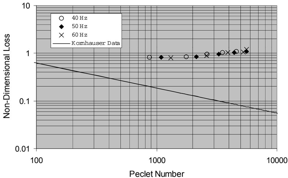
**Figure 5.** Compression Losses for the Ambient Cooler plotted non-dimensionally as a function of Peclet number. This is compared with an approximation to data from Kornhauser and Smith (ref 3, fig. 1) for the loss in a gas spring. The Peclet number is based on mean piston velocity, and the non-dimensional loss is based on the work of adiabatic compression.
