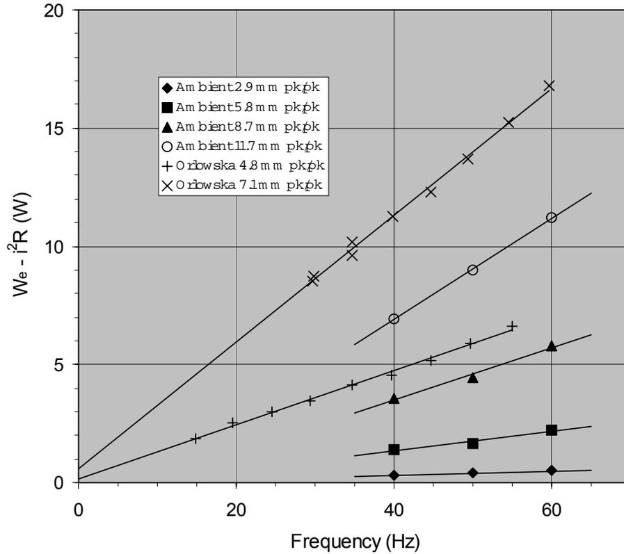
**Figure 2.** Compression Loss data for two Stirling coolers.
