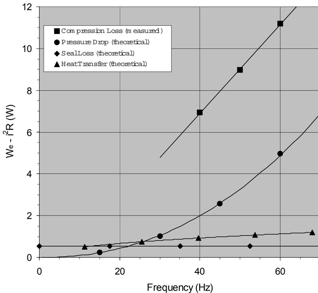
**Figure 4.** Measured Compression Loss for the Ambient cooler at 11.7 mm pk/pk stroke, compared with theoretical values for the expected loss mechanisms.
