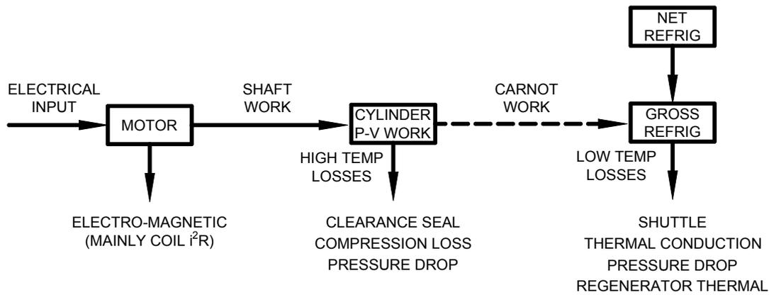
**Figure 3.** Schematic of Stirling Cycle Losses (simplified)
