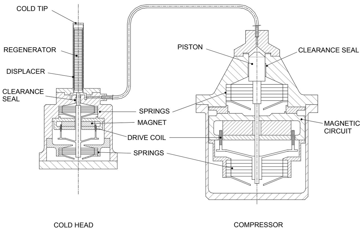
**Figure 1.** Schematic of original Oxford 'split' cryocooler
